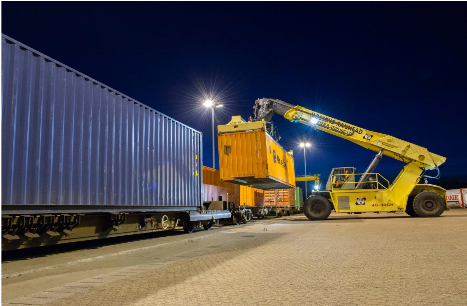
Figure 4.1- Reachstacker operating in a railport
